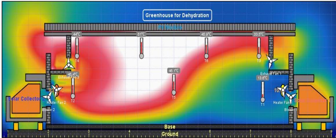
Figure 10: Simulation When Number of Heater Fan is One
