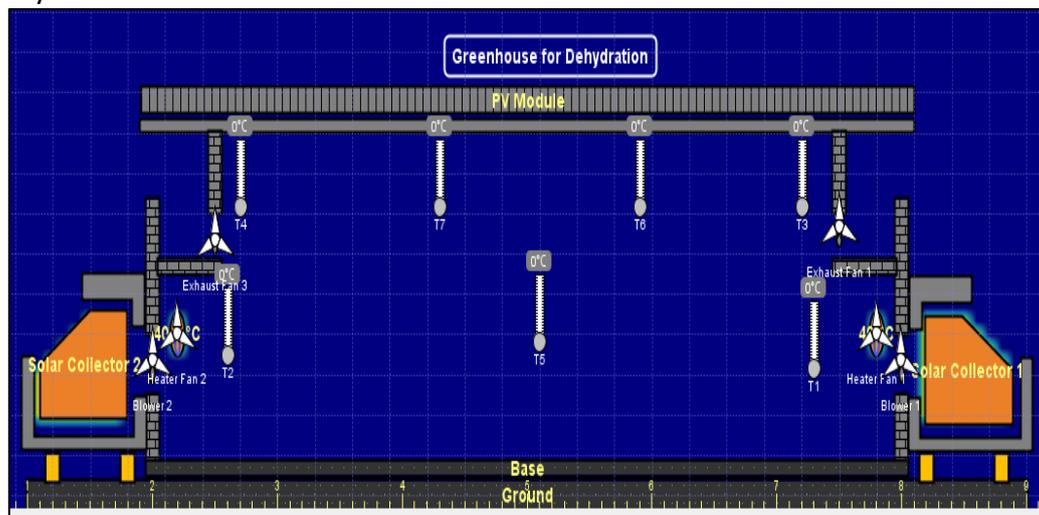
Figure 6: Greenhouse for Dehydration
