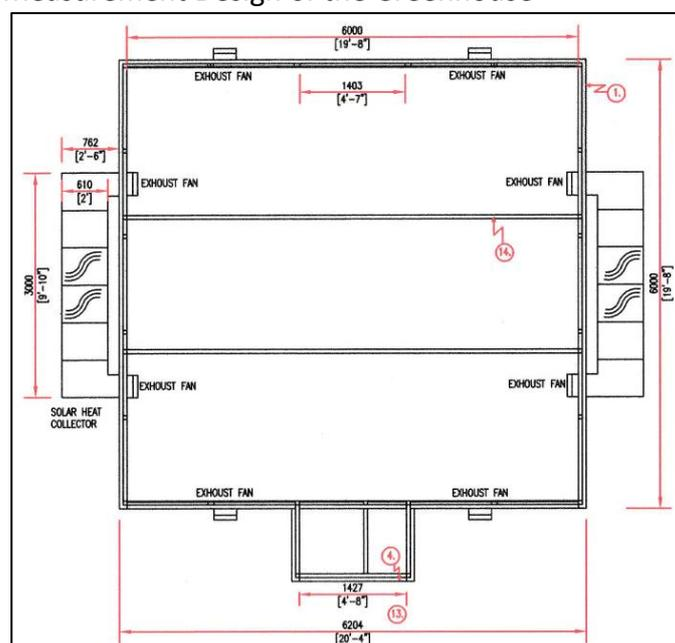
Figure 5: Top View Measurement Design of the Greenhouse
