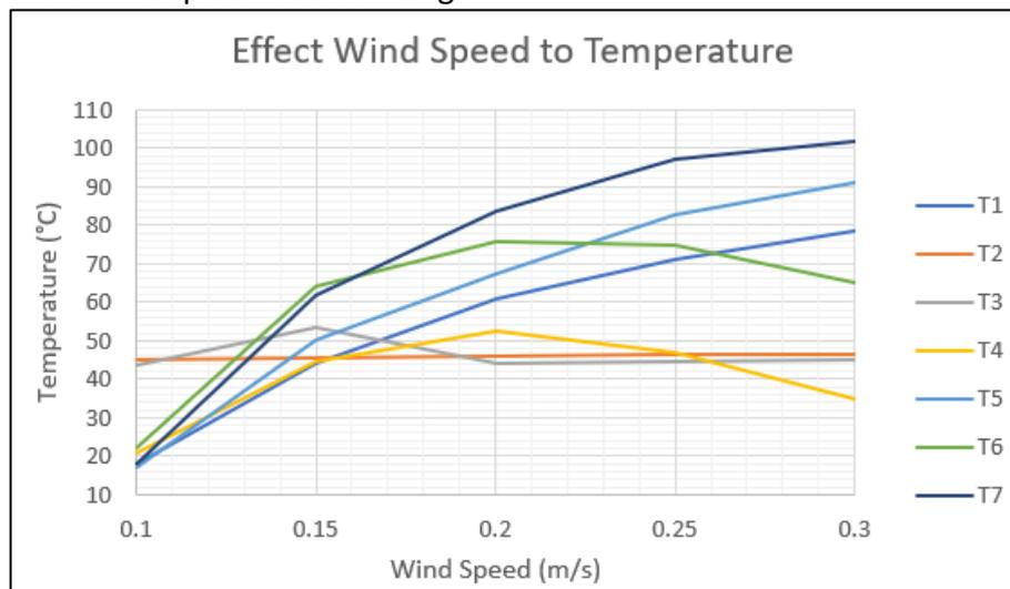
Figure 14: Effect Wind Speed to Temperature
