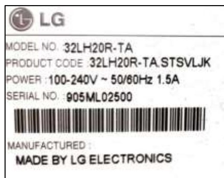
Figure 11: Television wattage specification
