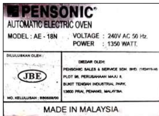
Figure 9: Electric oven wattage specification
