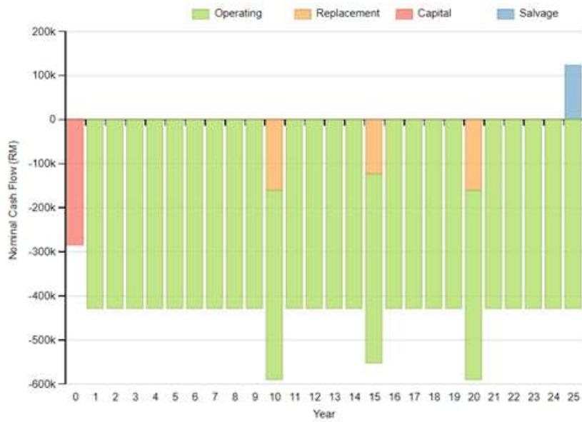
Figure 7: The cash flow of different cost type of the microgrid (Case 1)
