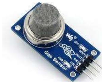
Figure 4: MQ135 Gas Sensor
