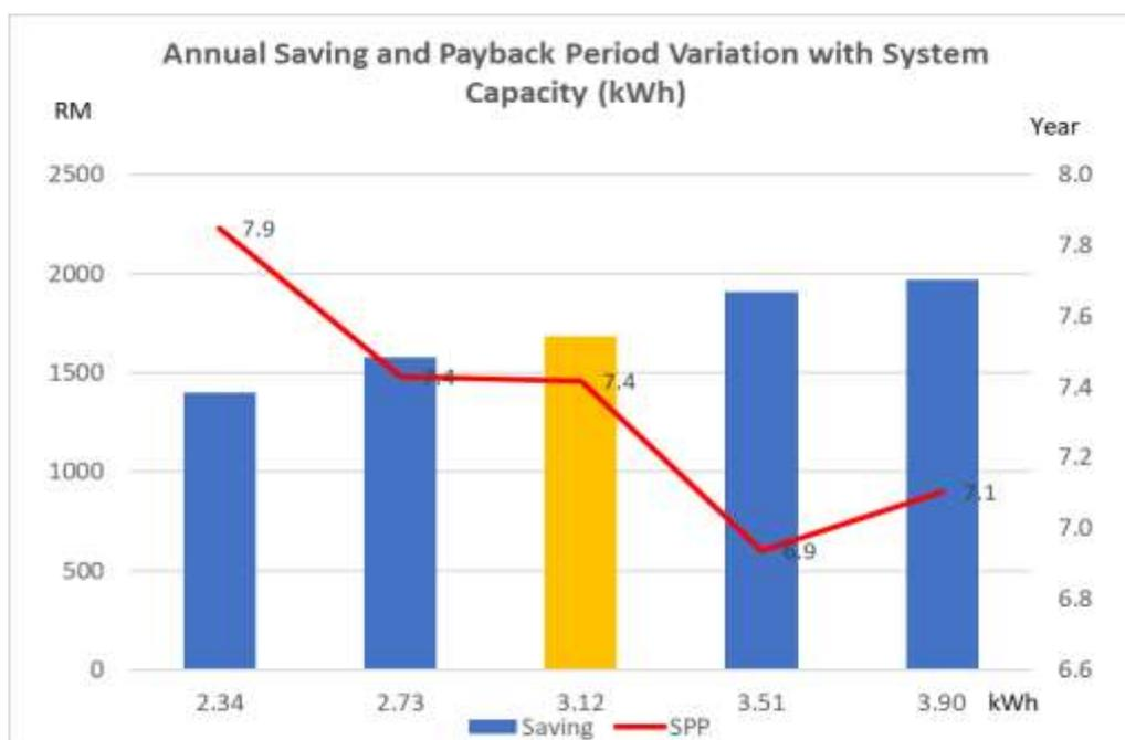
Figure 8. The variation of the annual saving and the payback period with the PV system capacity.
