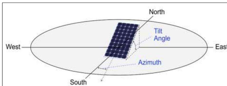
Figure 2. Roof orientation determines the tilt and azimuth angle.
