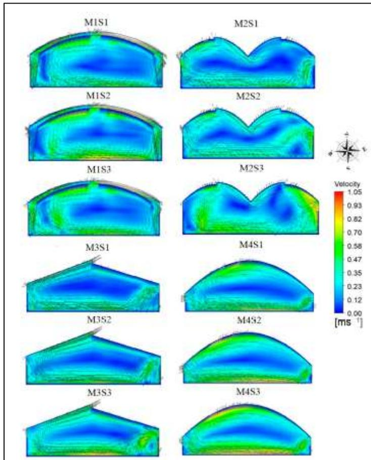
Figure 7: Air Flow of Thermal Distribution Inside Different Shape of Greenhouse Roof (Villagran et al., 2021)
