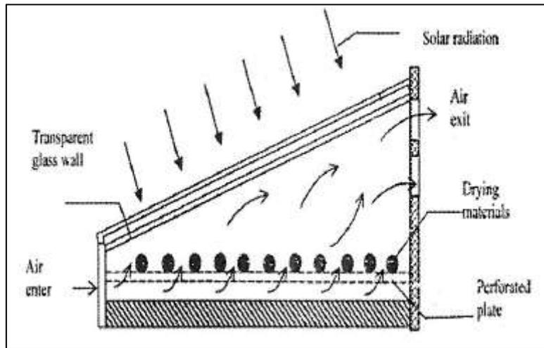
Figure 1: Passive Solar Dryer (Delfiya, 2019)
