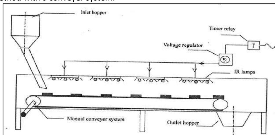
Figure 9: Infrared Dryer with Conveyor (Delfiya, 2019)
