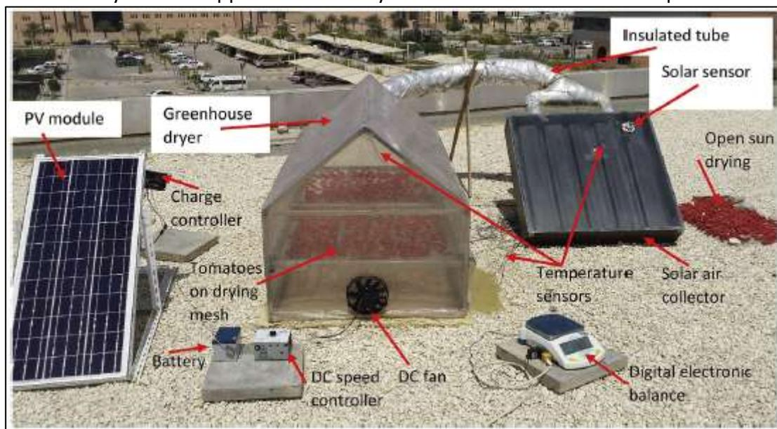
Figure 14: Greenhouse Prototype of the PV system with Solar Collector (Azam et al., 2020)
