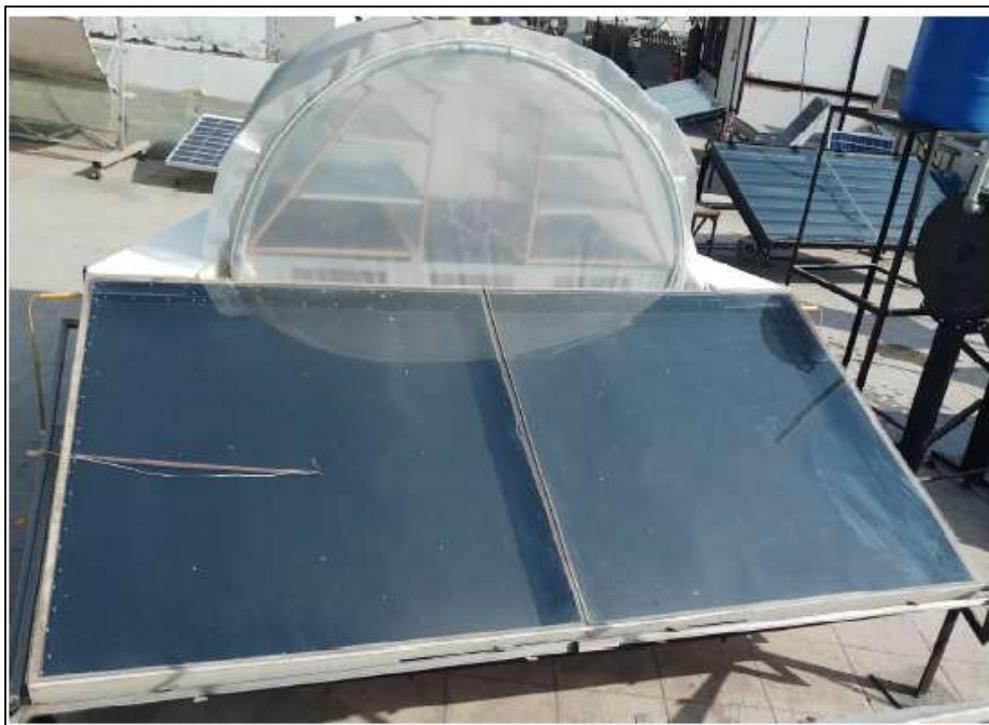
Figure 8: Prototype Tent-Type Solar Collector of Greenhouse (Mehta et al., 2018)
