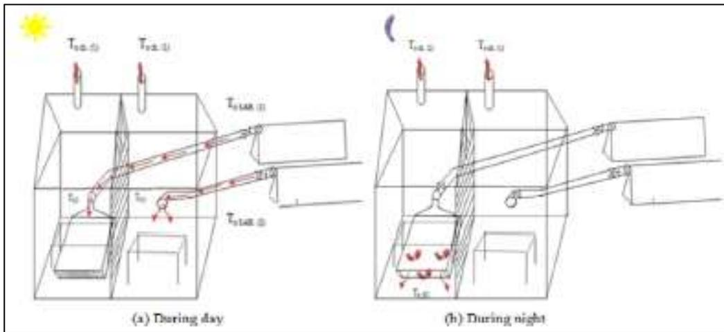
Figure 15: Principle of Heat Flow during Day and Night (Azaizia et al., 2020)
