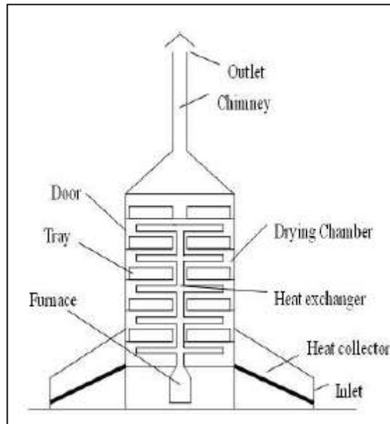
Figure 5: Hybrid Solar-Biomass Dryer (Yuwana et al., 2020)
