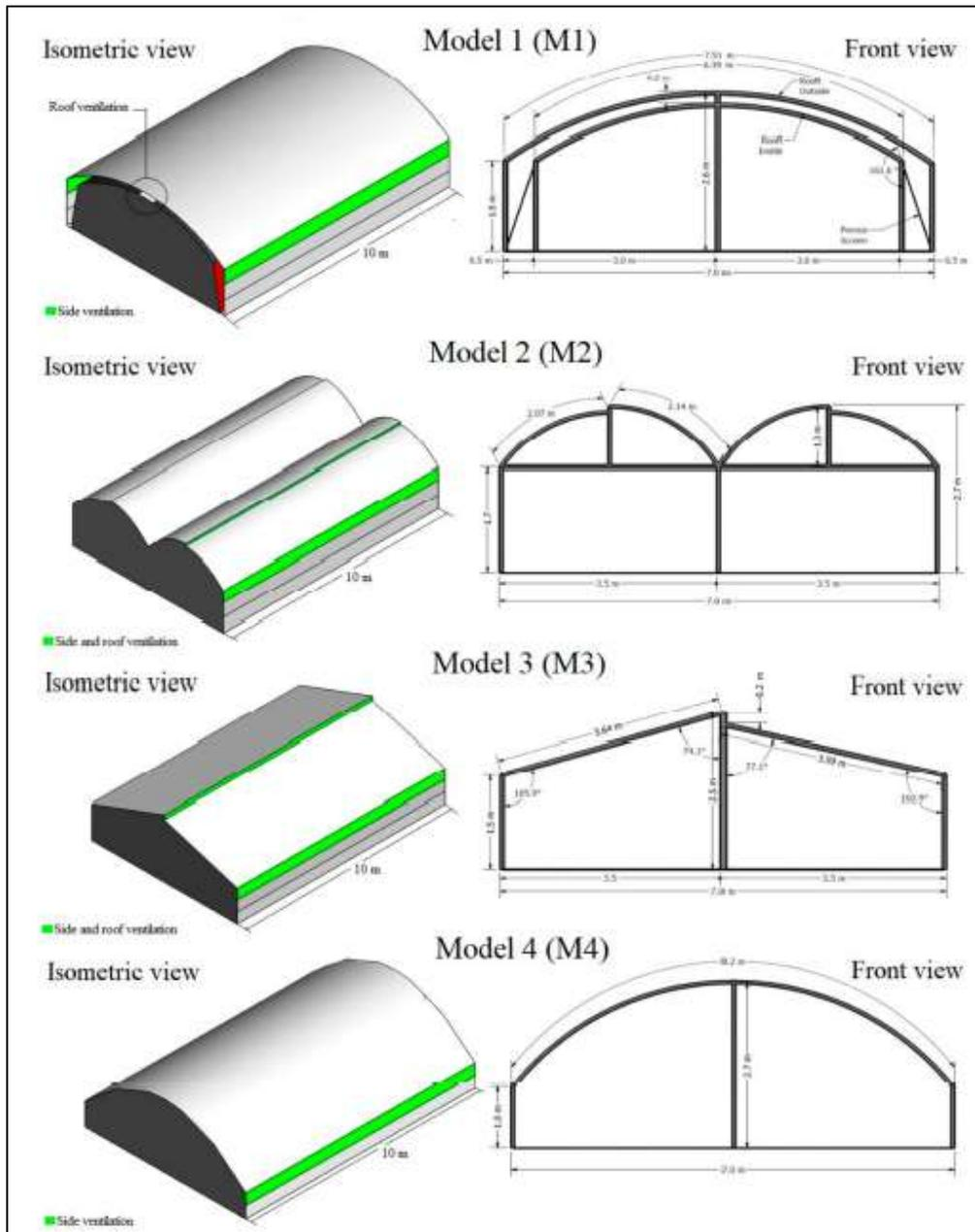
Figure 6: Different Types of Roof Shape for Greenhouse (Villagran et al., 2021)
