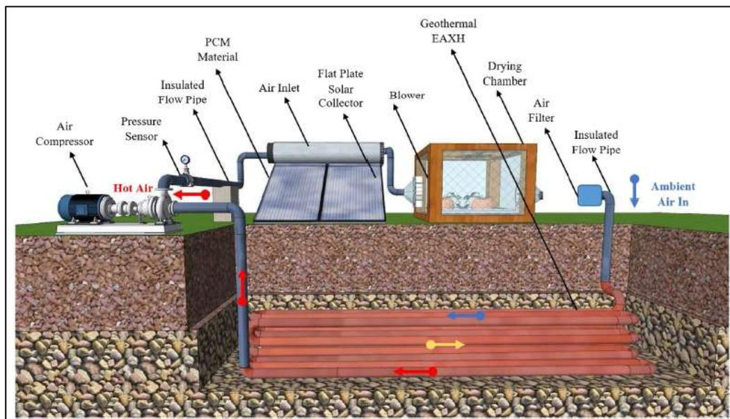
Figure 17: Concept Design of Geothermal PCM Solar Collector Greenhouse (Ananno et al., 2020)
