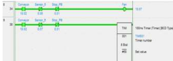
Figure 8. Running Program for Fan and stopping the overall system
