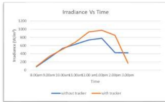
Figure 11: Irradiance Vs Time comparison graph.
