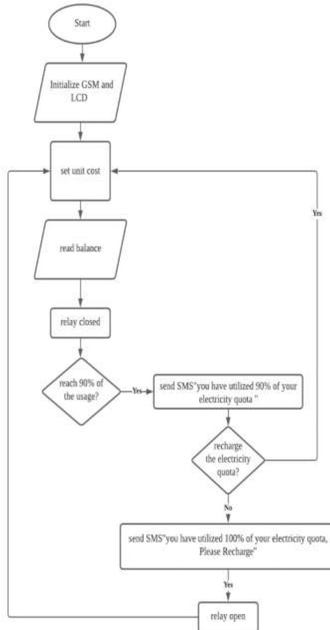
Figure 2: Flowchart for prototype single-phase prepaid energy meter
