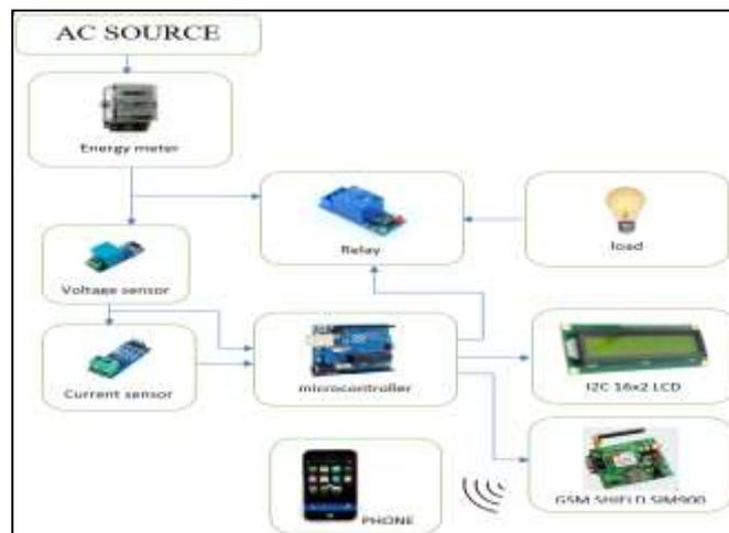
Figure 6: Block diagram of prototype Prepaid Energy Meter.
