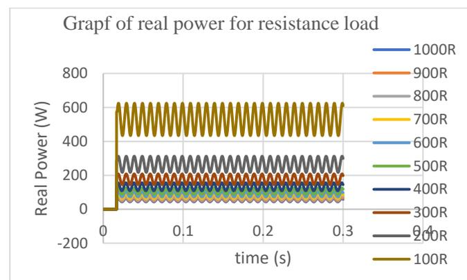
Figure 9: Varied active power between resistance of 100 Ω to 1000 Ω
