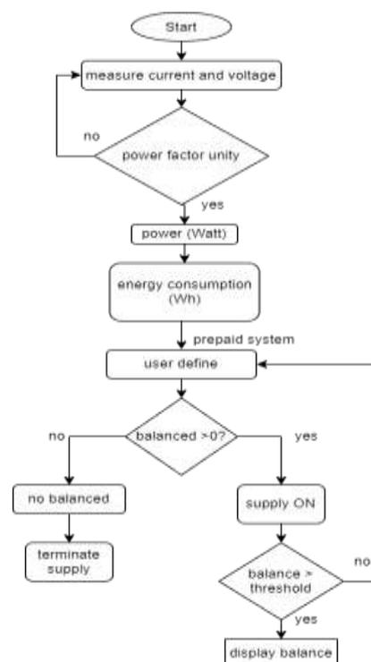
Figure 1: Flowchart for modeling single-phase prepaid energy meter using MATLAB/Simulink.
