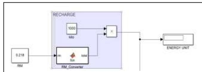
Figure 5: Recharge Ringgit to Energy unit Converter Subsystem
