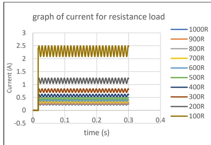
Figure 8: Varied current between resistance of 100Ω to 1000Ω
