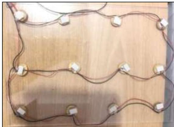
Figure 3: Connection of Piezoelectric Footsteps
