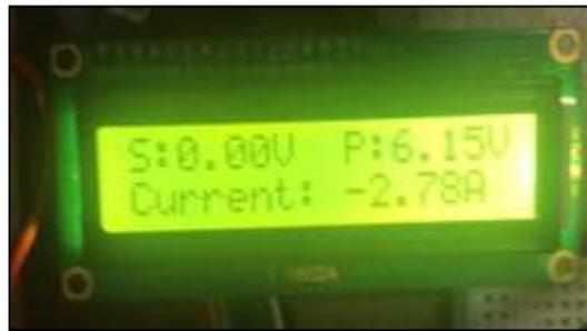
Figure 11: Reading when no presence of solar energy and pressure on footsteps is applied
