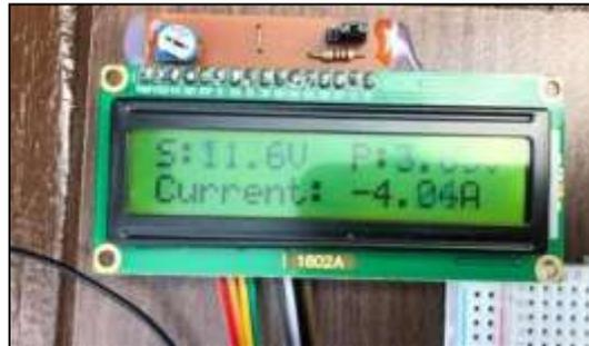
Figure 15: Reading when prototype placed under hot sun at 12pm and pressure applied on piezoelectric footsteps board
