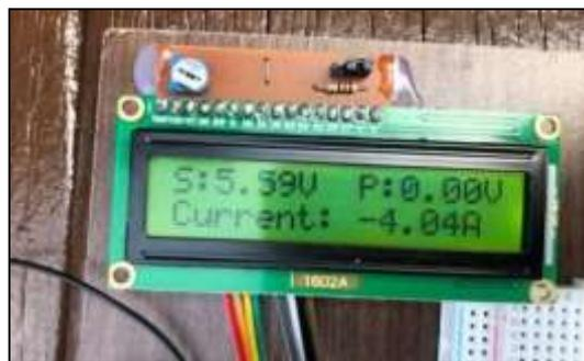
Figure 13: Reading when no pressure applied on the footsteps and presence of solar energy
